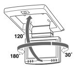
**Tip**Before closing the display monitor, make sure that the monitor is turned and facing the enclosure (you will hear a click).
